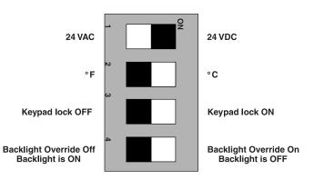
Figure 3: RAK163P1 and RAK147P1 Factory Default DIP Switch Settings
